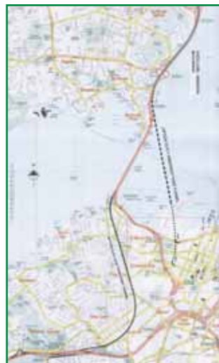
Figure 12. Option III – Immersed-tube tunnel and Ponsonby tunnel
